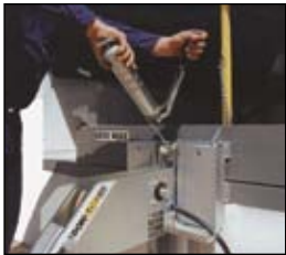
E-Z-Lube™ axle design makes occasional lubrication quick and simple.
